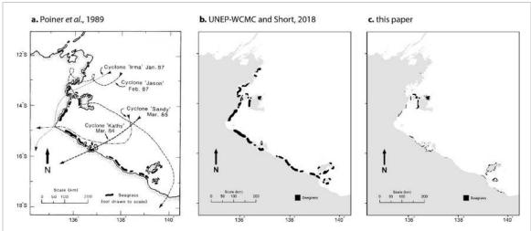
Figure 5. Example of data migration from 'not drawn to scale' sketch to GIS: (a) hand-drawn source (reprinted from [34], copyright (1989), with permission from Elsevier) (note 'not drawn to scale'); (b) digitised into WCMC database, and; (c) revised polygons from 'to scale' surveys. On average, meadows in 'not drawn to scale' source extended 10 km from shoreline, however in 'to scale' survey, meadows rarely extended greater than 1 km from shoreline.
