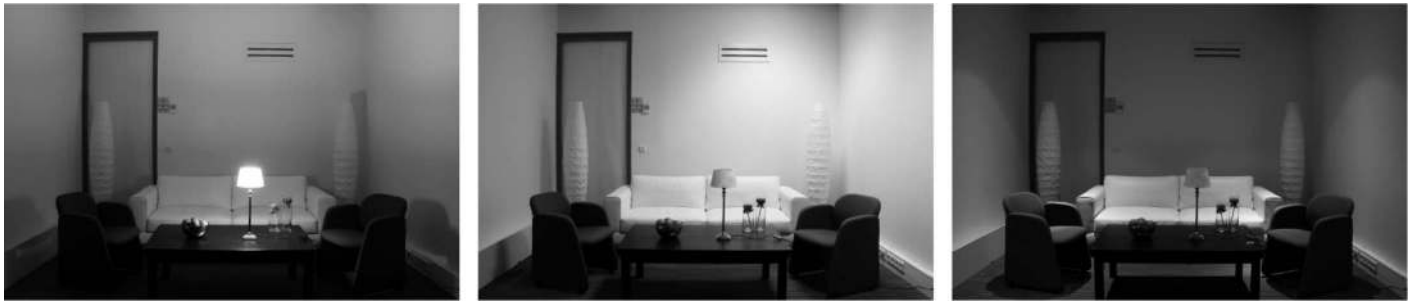
Figure 1. Light conditions: visible light source (LAMP), diffused light sources in the ceiling on the right side of the scene (DIFFUSE), two collimated light sources in the ceiling, one on the left and the other on the right side of the scene (SPOTLIGHTS).
