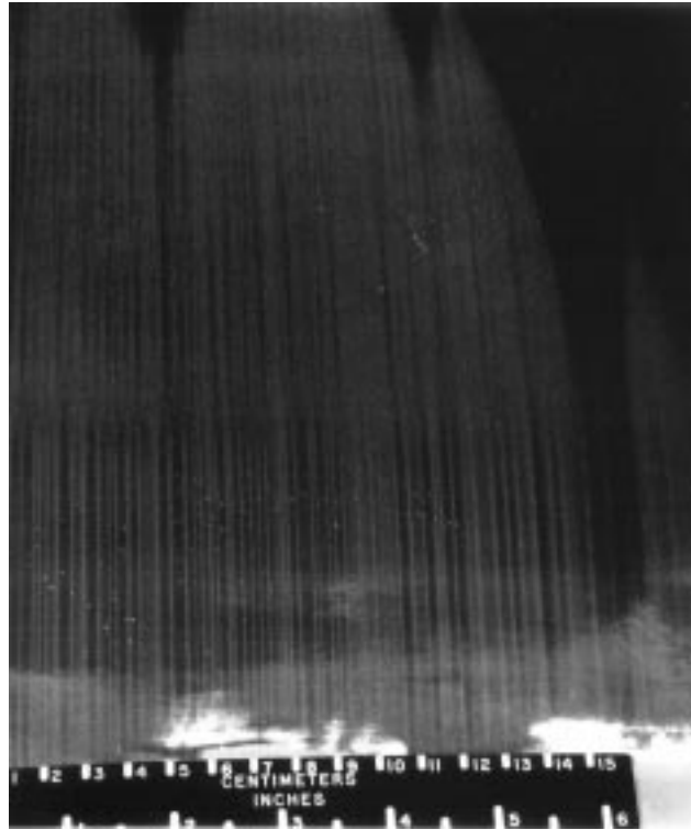
Figure 4(b).- Flow visualization using sublimating chemicals M_\infty = 0.075 , R_c = 3.21 \times 10^6 .
