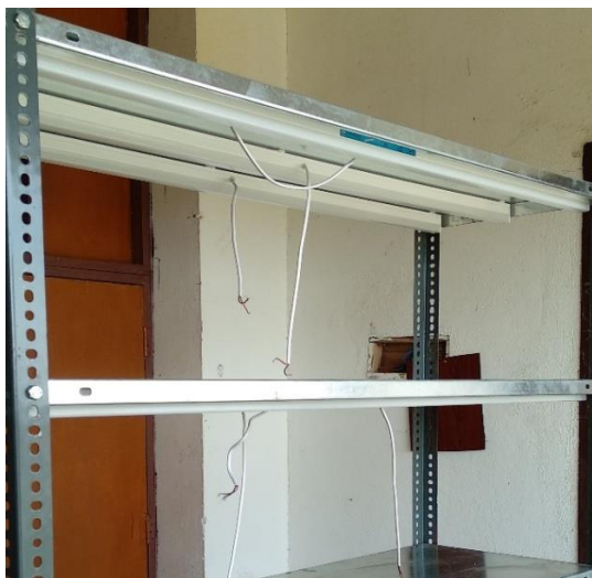
Fig.1. Rack system with T5 Grow Lights
