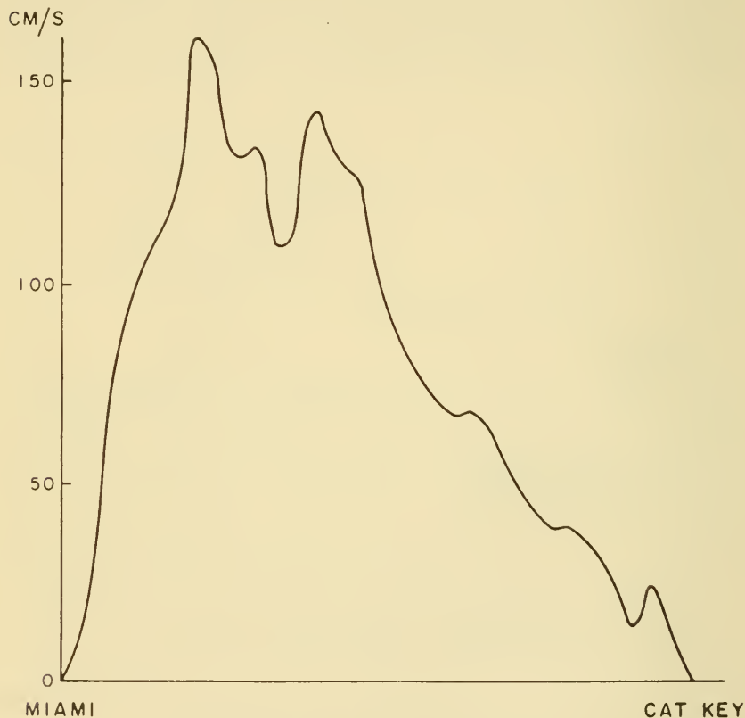
Fig. 71. Sample surface velocity profile of the Florida Current between Miami and Cat Key, according to Murray's (1952) towed-electrode measurements.
