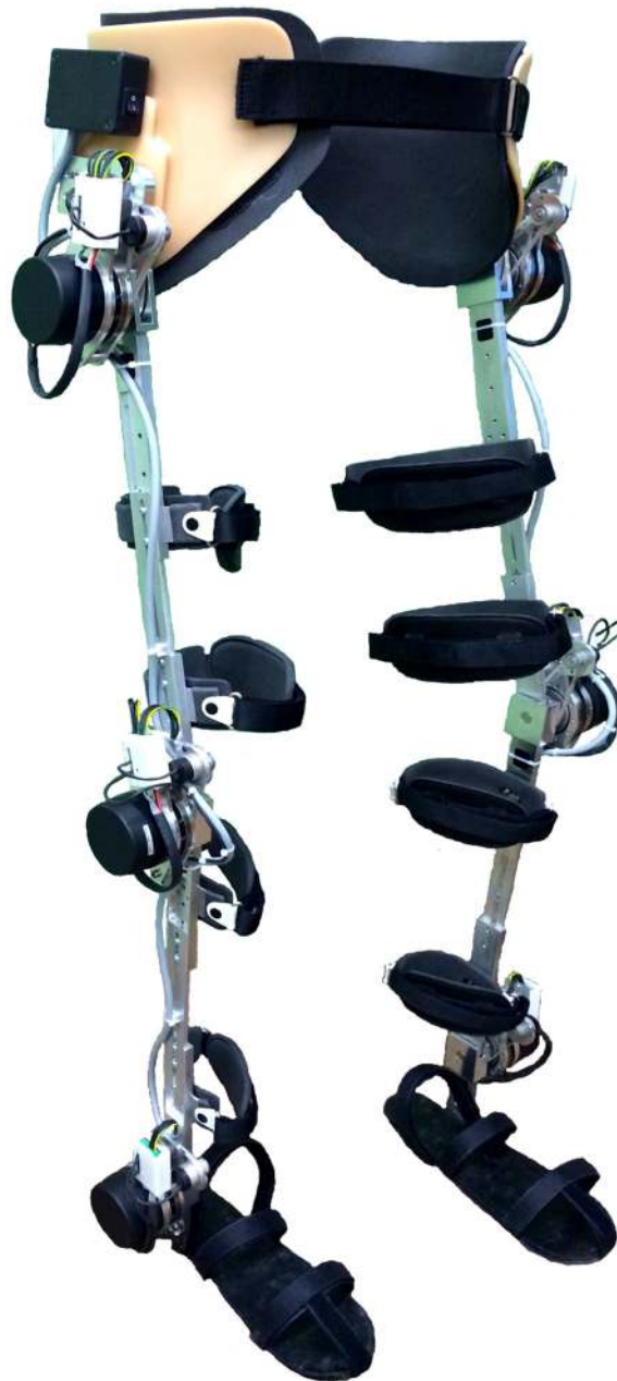
Fig. 1 H2 robotic exoskeleton. The six joints are powered by brushless DC motors coupled to Harmonic Drive gearboxes. All sensory information comes from sensors placed on the exoskeleton: 6 potentiometers, 18 Hall Effect sensors, 24 strain gauges and 4 foot switches. A rechargeable battery pack of lithium polymer powers the exoskeleton
