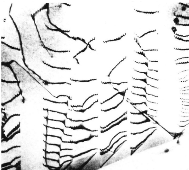
Figure 9 Bright-field TEM image of 304 stainless steel at a strain of 0.8%. Grain boundary ledges are visible. From [52].
