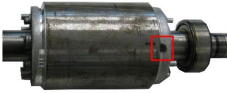
Fig. 3. Rotor of the tested motor with a forced broken bar fault.
