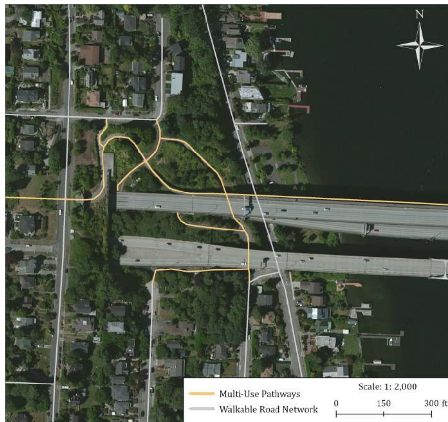
Fig. 3 Example section of the “pedestrian-enhanced” walkable road network that excludes freeway road segments while integrating multi-use pathways. ©2019 Urban Design 4 Health, Inc
