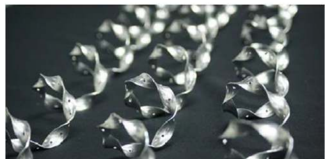
Fig. 15. Perforated helical twisted tapes (Nanan et al., 2014).
