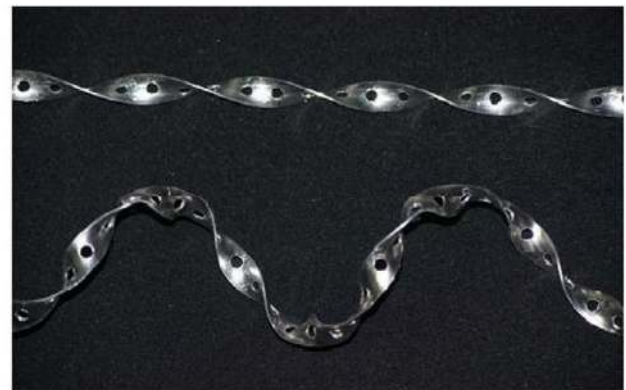
Fig. 13. Isometric, front and top view of helical twisted tape (Nanan et al., 2013b).
