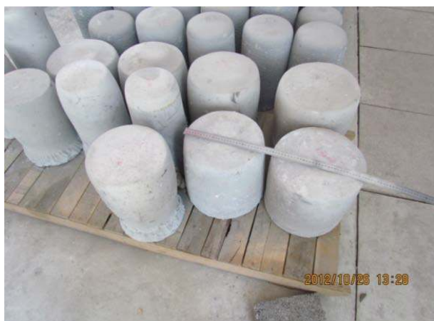
Figure 1. Billets of Al alloy by spray forming.
