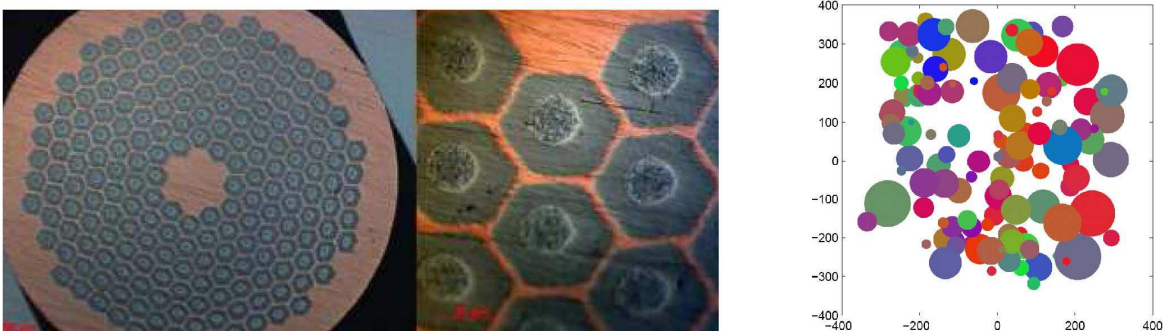
Fig. 5: First tomogram at HEMS of a Nb 3 Sn superconductor with scan volume 1 mm 3 at 70 keV (left), first centre-of-mass grain map of undeformed Al at 60 keV (right) – 14 cuts á 50 \mu m, measured with beam size of 0.05 x 1.0 mm 2 . 128 indexed grains are shown as spheres with diameters reflecting relative volumes and colours corresponding to orientation (position accuracy 30 \mu m, orientation accuracy 0.15 o , relative error of volume 35 %, courtesy J. Oddershede).
