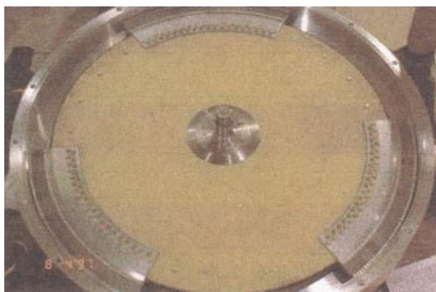
FIG. 6. (Color) Photograph of the PST chopper with the front casing removed. The chopper disk and the three cassettes which contain the HOPG crystals are exposed. The distance between the axis of rotation and the center of the crystals is 505 mm.
