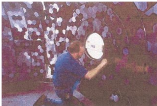
FIG. 12. (Color) Photograph of the HFBS analyzer with technician S. Slifer kneeling to inspect the alignment.
