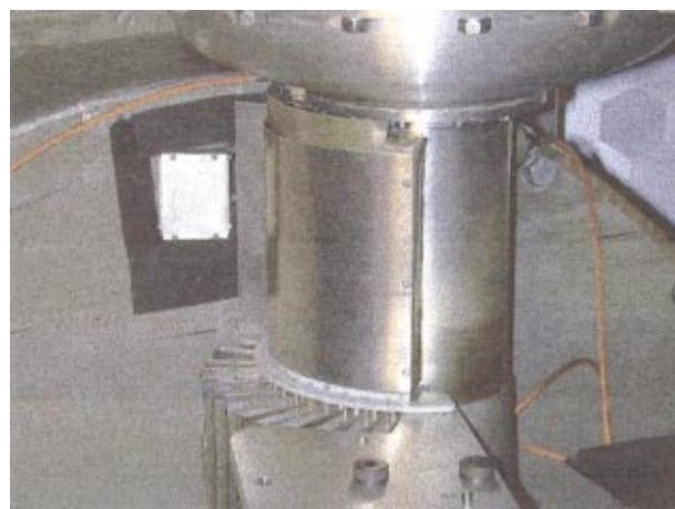
FIG. 14. (Color) Picture of the HFBS sample area as viewed from inside the large vacuum chamber, which houses the PST chopper, analyzer, and detector assembly.
