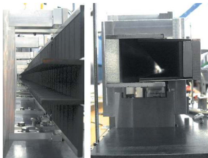
Figure 8 (Left) Vertical and horizontal absorber plates of \text{B}_4\text{C} , designed to avoid the focusing in the GISANS mode of MARIA. (Right) The absorber plates are moved into the vertical elliptical NG and form together with the slits S1 and S2 a tunnel for the double-collimated neutron beam.
