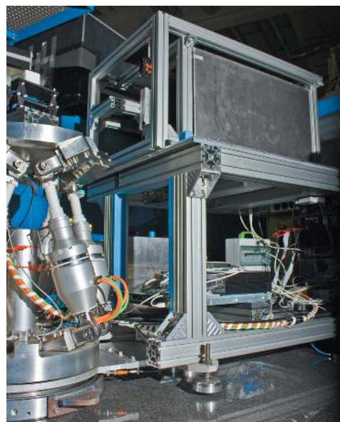
Figure 9 View of the open detector arm with the ^3\text{He} SEOP wide-angle spin filter installed and a glimpse on the hexapod at the sample position.
