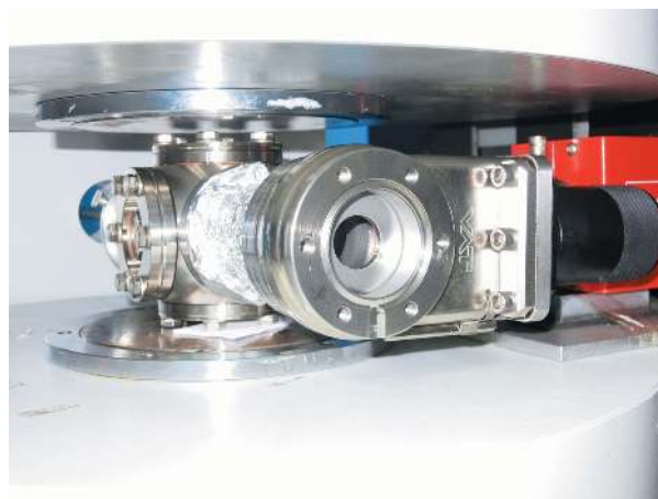
Figure 13 The versatile UHV transfer chamber that bridges the production of the sample inside the MBE system and the measurement at MARIA. The transfer chamber is placed inside the electromagnet and the exit window of the beam is at the centre of the photograph. On the left hand side is a window for the pre-alignment of the sample with a laser, and on the right hand side the red getter pump is visible.
