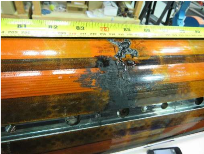
Figure 28. The short coil to heater in MQXFAP1.
