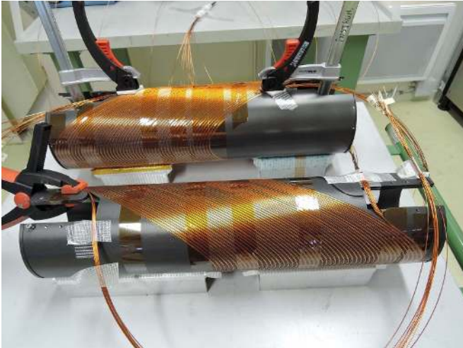
Figure 52. Two two-tilted solenoids of the short model of the canted corrector before being inserted one into the other.
