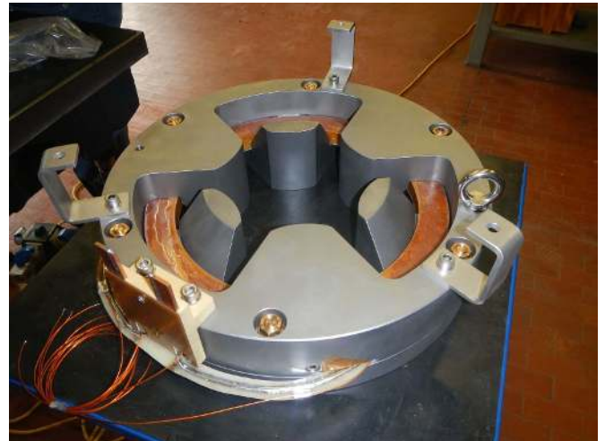
Figure 68. The final assembly of the sextupole corrector based on round coil superferric design and MgB 2 conductor.
