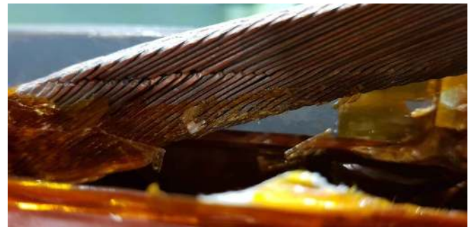
Figure 44. The damaged magnet lead after disassembly in MBDRS1.
