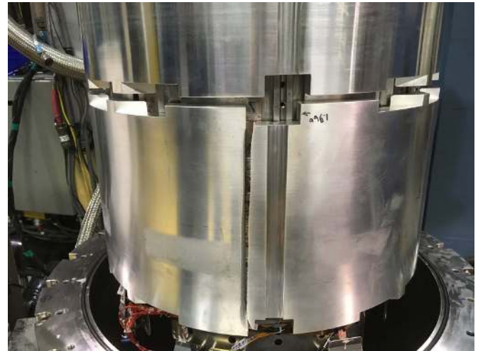
Figure 29. The broken shell in MQXFAP2.
