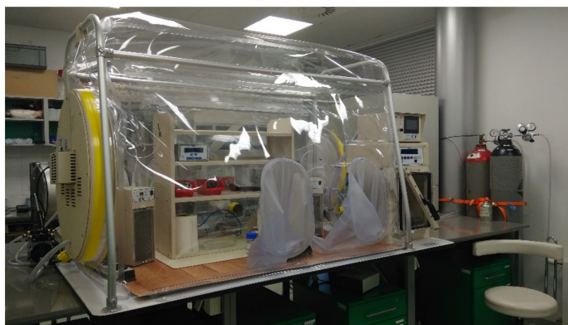
Figure 3. Anaerobic box (Coy Laboratory Products, USA) (Photo: Laboratory).
