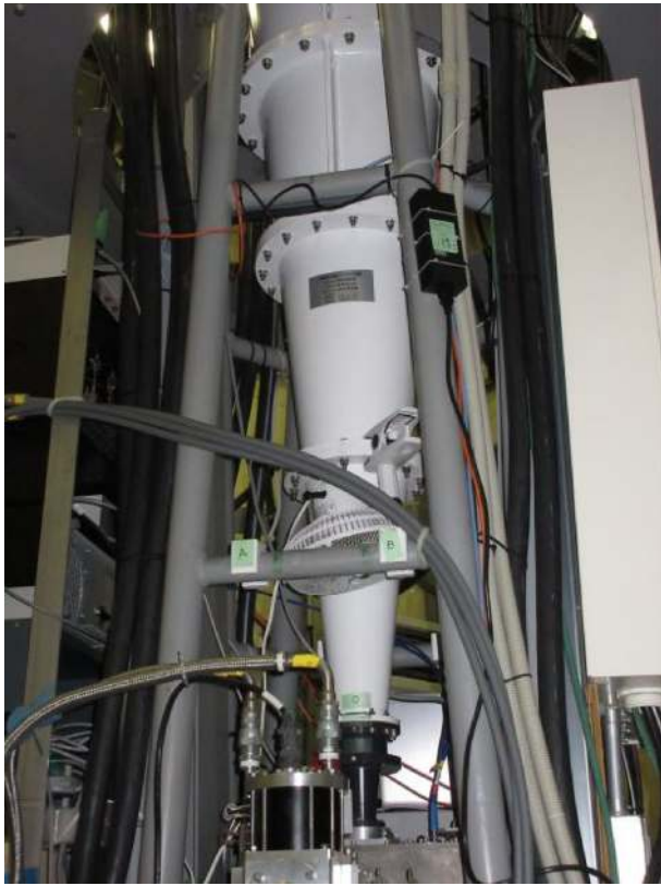
Fig. 3. Photograph of the feed horn. By exchanging the bottom of the feed horn, we can change the observation band. (Color online)
