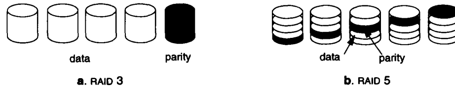
Fig. 1. Data and parity layout for two different RAID levels.
