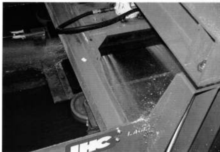
Figure 10.11: 2:1 fender with bearing thickness 5 mm (view II).
