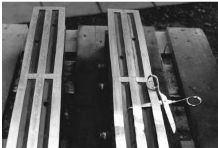
Figure 10.8: 10:1 fender with bearing thickness of 0.8 mm. The bearing is bend outward and the bonding between the bearing and the support has failed.
