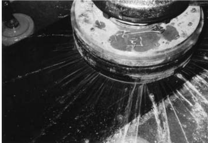
Figure 2.5: Testing of the hydro-foot. These tests have been carried out above water and the water supplied to the bearing can be seen squirting out.
