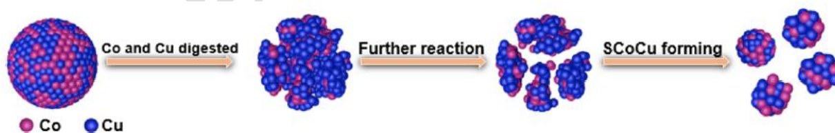
Figure 35. Schematic illustration of the fabrication strategy of the SCo/Cu Alloy. Reprinted with permission from ref 180. Copyright 2020 American Chemical Society.
