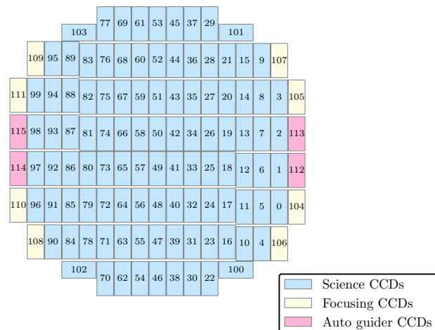
Fig. 1. The layout of 116 CCD chips, each of which has 2048 \times 4096 pixels ( 5.73' \times 11.47' ), on the focal plane. The CCD chips are arranged with two different gaps of approximately 12'' and 53'' between the neighboring chips. The focal plane is approximately 1.5^\circ in diameter. There are 104 science chips (indicated in blue), 4 chips used for auto-guiding (in yellow) and 8 chips for monitoring the focus (in light red). Each chip is identified with a number from 0 to 115.
