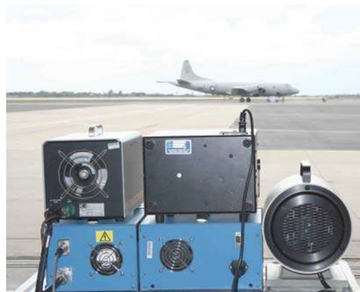
Fig. 5. Calibration Setup using Multiple Blackbody Radiation Sources
