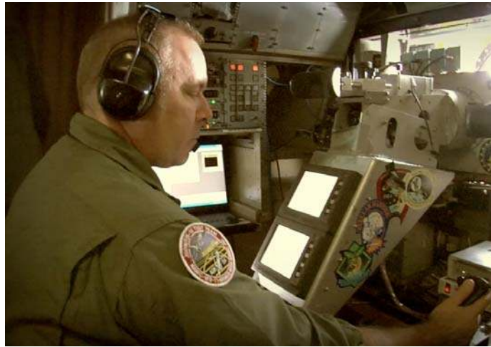
Fig. 6. Cast Glance Operator Configuring the NIR Detector for Optimal Response
