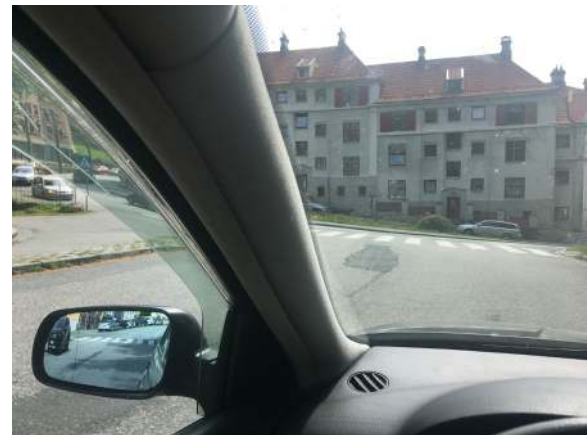
Fig. 3 The A-pillars next to the windscreen can hide the view of other road users
