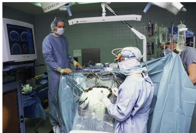
Fig 1. Image-guided system for brain surgery showing the optical tracking system at the top right and the display overlay on the far left . The patient is under the blue cover in the middle . (Photograph courtesy of Richard Bucholz, MD, St. Louis University).
