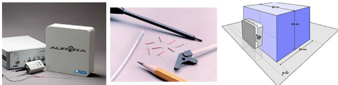
Fig 2. Aurora electromagnetic tracking system components, sensors, and measurement volume. The left picture shows (from left to right) the control unit, sensor interface device, and electromagnetic field generator. The middle picture shows the sensor coils (red objects in the middle of the figure). The right picture shows the measurement volume which is a 500 mm cube starting 50 mm from the front of the field generator (Image courtesy of Northern Digital, Inc.).
