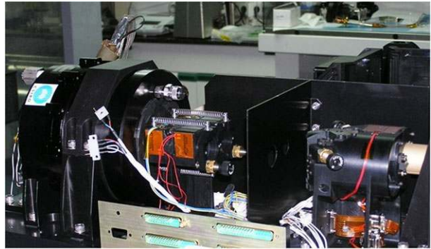
Figure 3 The temperature-controlled side of the IMaX optical bench including the pre-filter and LCVR mounting (right), the collimator and camera lenses mounting, and the etalon TCPE (left). The stray-light baffle is seen in between the two first elements.
