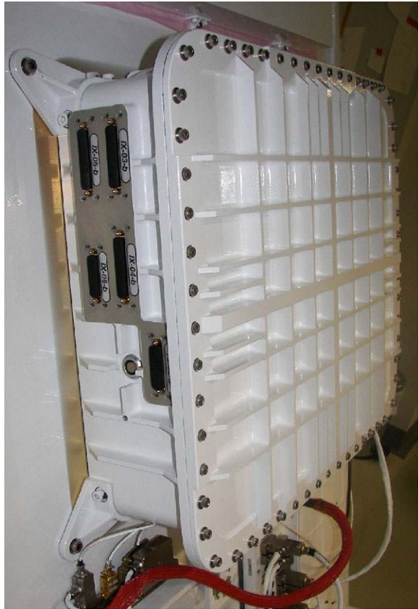
Figure 10 The pressurized IMaX MEE mounted into the flight panel.
