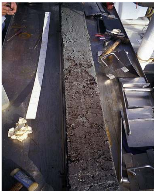
Fig. 1 Photograph of a 1.5-m-long sediment core taken in 22 m water depth at the Russell Island group (Latitude 17° 13.5' S, Longitude 146° 05' E) on the Great Barrier Reef Shelf in February 2003. Note the abrupt demarcation halfway up the core between brown mangrove peat and more recent fine carbonate gray sand. Mangrove peat on the shelf is typically aged at 9.3–9.1 ka BP [87]
