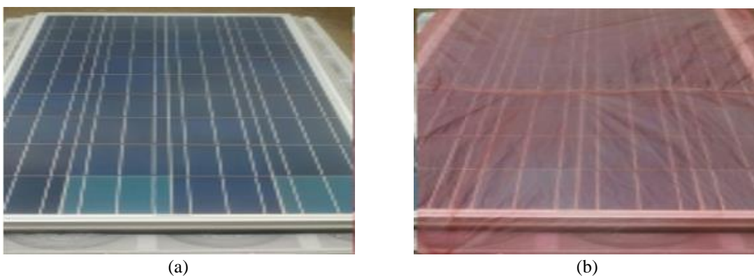
Figure 2. Photovoltaic module without filter and with red coloured filter respectively, (a) a photovoltaic module without filter, (b) photovoltaic module with a red filter
