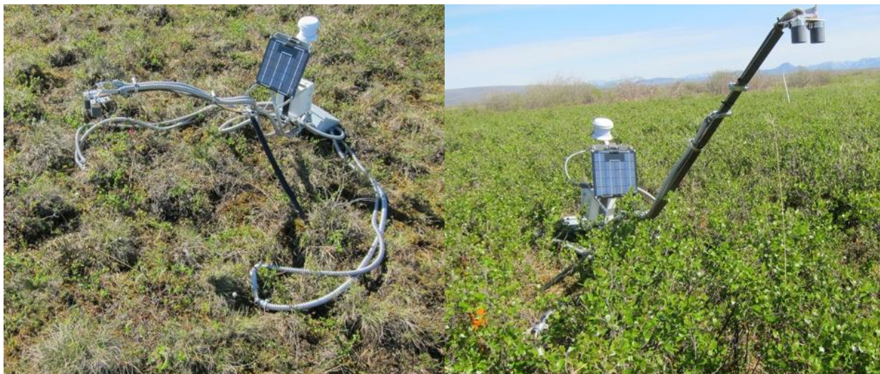
Figure 2.4. Example of equipment assemblages in evergreen/graminoid (EG) canopy (left) and deciduous shrub (DS) canopy (right) used in this study to determine the normalized difference vegetation index (NDVI). Sensors collected photosynthetically active radiation (PAR), solar irradiance, and air temperature data every two-minutes from 1 June to 5 September 2013.
