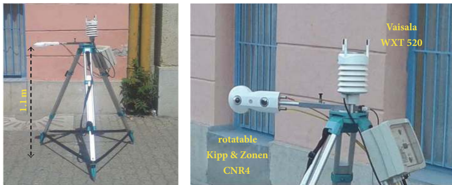
FIGURE 3: One of the human-biometeorological stations used in this study (photo taken at P3 site).
