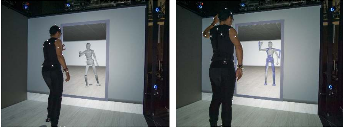
Figure 1: Left: The basic virtual mirror scenario consists of an empty room and a simplistic mirror avatar. Right: The extended scenario employed in the experiment, where the target movement is shown by a semi-transparent blue “ghost character”.
