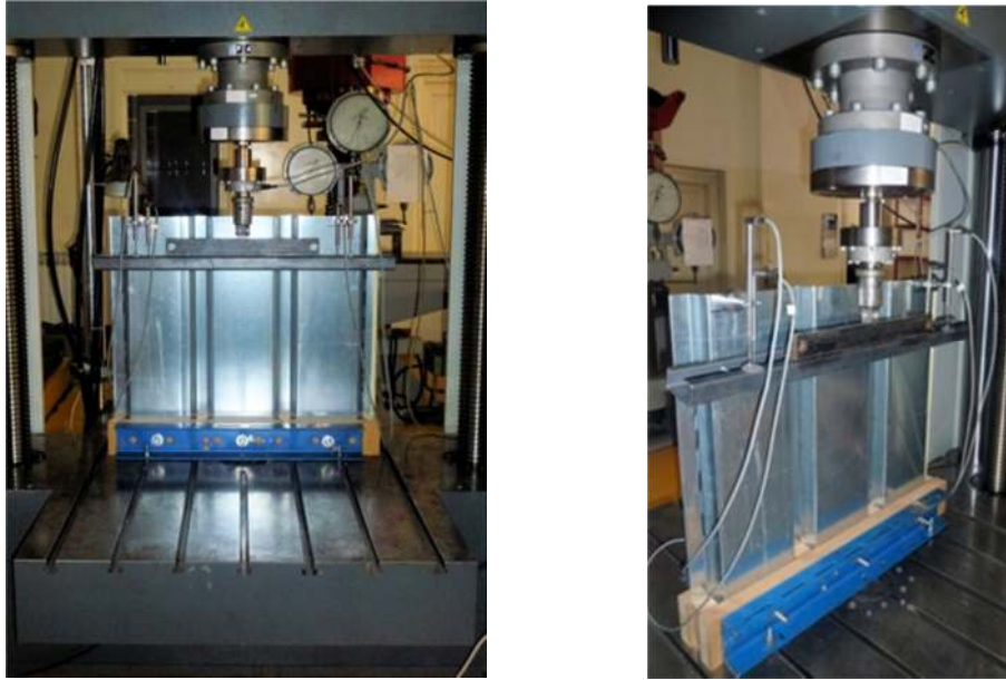
Fig. 5 Determination of rotational stiffness of the rotation spring
