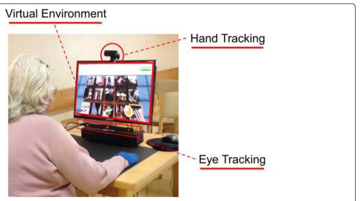
**Fig. 1** Experimental setup. The setup includes an eye-tracker, hand tracker and a virtual environment displayed on a high-resolution display monitor. Patients interact with the system through arm movements on a flat surface
