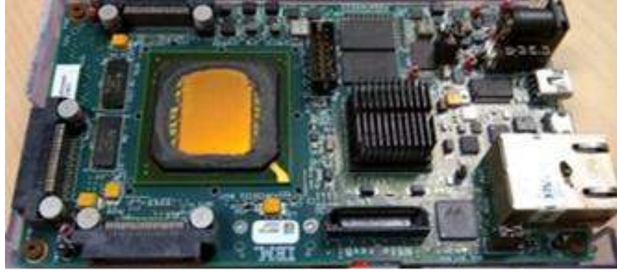
Fig. 6. Picture of the TrueNorth board after the chip (middle-left) was delidded.
