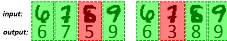
Fig. 9. Example of how changes can occur due to radiation without affecting the overall classification accuracy. The left side is the pre-irradiation classification of the digits 6, 7, 8, and 9, and the right side is the same digits after irradiation to a fluence of 5.6 \times 10^7 \text{ cm}^{-2} .
