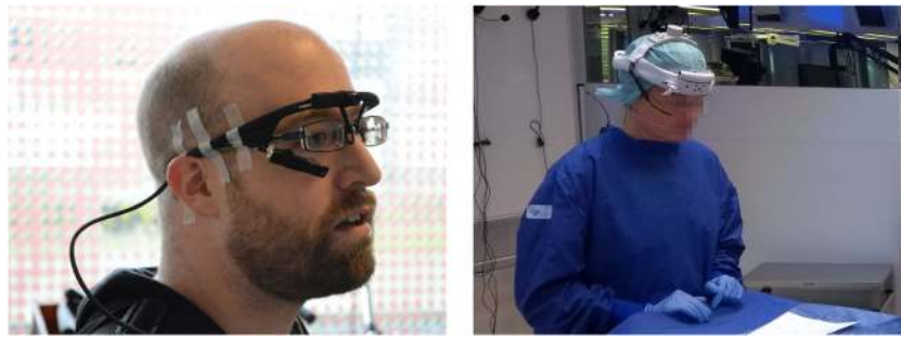
Fig. 1 Head-worn eye trackers. Two examples of extreme measures taken by researchers to prevent slippage of a head-worn eye tracker: tape ( left panel , courtesy of Jeroen Benjamins) and a helmet mount ( right panel , courtesy of Shahram Eivazi)
