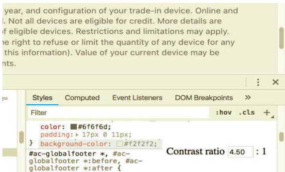
Fig.18. Applying WCAG 2.0 Level AA minimum contrast ratio 4.5:1 on Apple.com official home page
