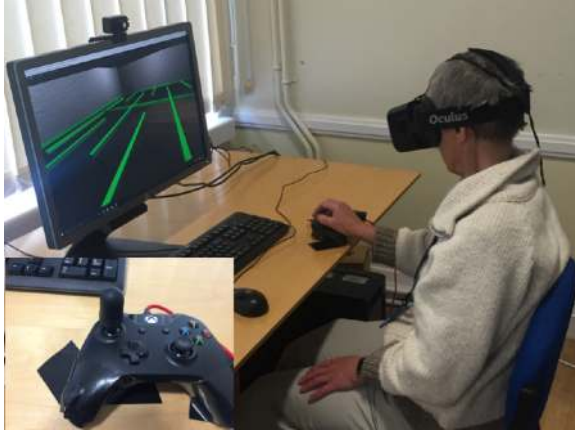
Fig. 4. The Wheelchair-VR Hardware components consist of the PC, an Oculus Rift DK2 HMD, and an Xbox controller. Insert shows the adapted joystick on the Xbox controller.
