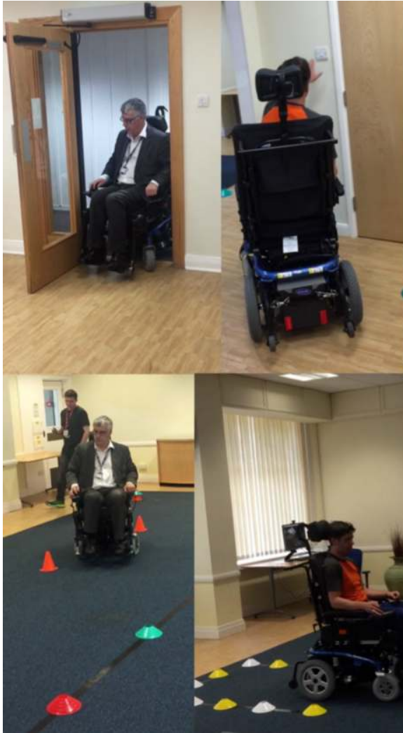
Fig. 5. The four components of the timed obstacle course. Top left: go through doorway. Top right: traverse a circle and reach out to press a light switch. Bottom left: slalom. Bottom right: reverse parking.
