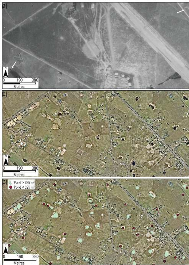
Figure A1. Historical changes in pond distribution from a 2.7 km 2 area in south-east Queensland, Mt Tarampa (27°27'44" S, 152°28'59" E). (a) 1944 aerial images showing 2 ponds indicated by white arrows, (b) 2017 aerial image showing 54 ponds and (c) showing the relative distribution of ponds from the Reservoir (> 625 m 2 ) database and the Water Storage Point (< 625 m 2 ) database – together this results in a density of 20 ponds km -2 .
