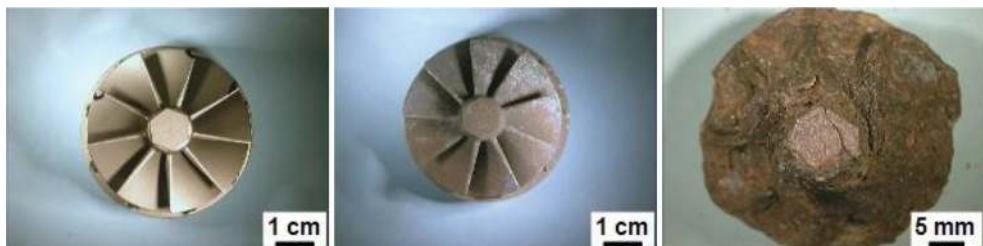
Figure 20. Macroscopic images of the second untreated TiAl rotor with a different chemical composition before (a), after 100 h (b), and totally destroyed after 1200 h (c) of oxidation at 1050°C in laboratory air.
