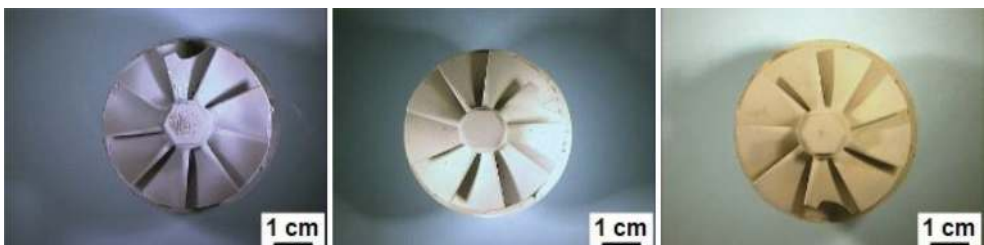
Figure 21. Macroscopic images of an F-treated turbocharger rotor after spraying (a), after 100 h (b), and 1200 h (c) of oxidation at 1050°C in laboratory air.
