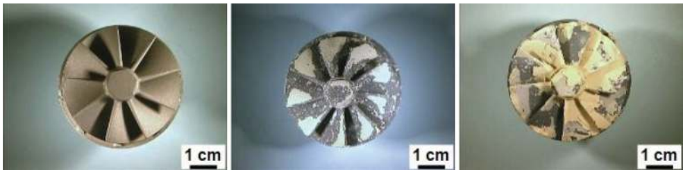
Figure 19. Macroscopic images of an untreated turbocharger rotor before (a), after 100 h (b), and 1200 h (c) of oxidation at 1050°C in laboratory air.
