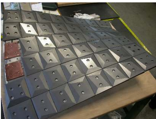
Fig. 4. Heat shield with clamped graphite tiles, two tiles on the left inside are removed to view CuCrZr plates of the 3D-shaped cooling structure. Every tile is differently machined with facets according to physics specification. Screws are made of TZM.
