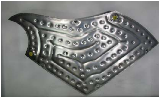
Fig. 5: Wall panel, seen from the backside. The internal cooling structure is clearly visible.
