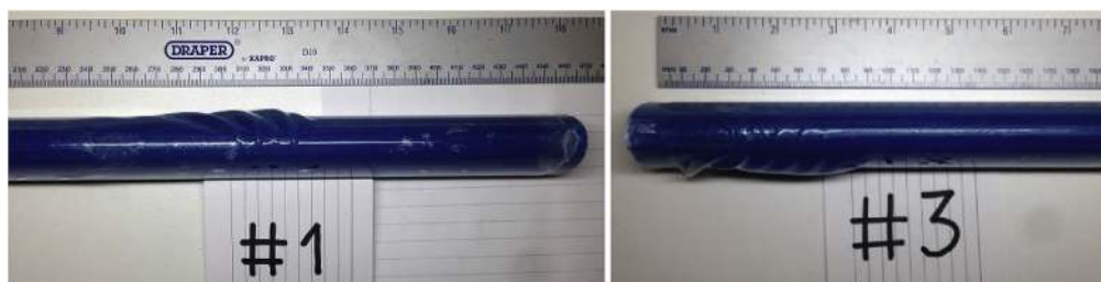
Fig. 9. Significant tape detachment and water entrapment in sample 1 after 8 h (left) and in sample 3 after 5 h (right) of rain erosion testing.
