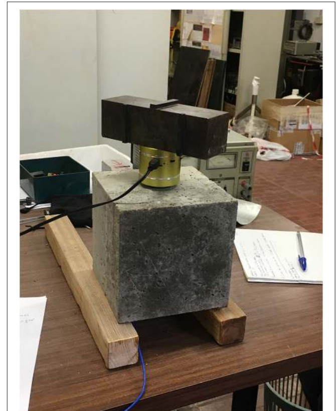
FIGURE 3 | Experimental setup, showing a metaconcrete specimen, the two transducers, and the vibration speaker pressurized with a weight to increase adherence.
