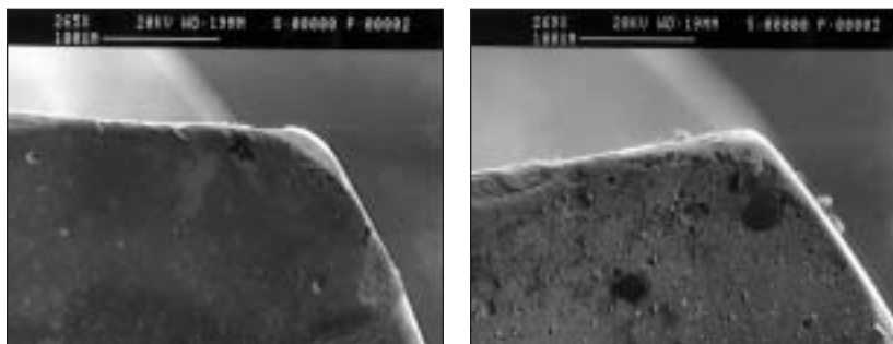
Fig 8 SEM of Paragon drills following test completion. (Left) Second 2-mm drill; (right) a 3-mm drill. Cutting edges do not show blunting as in Fig 7.
