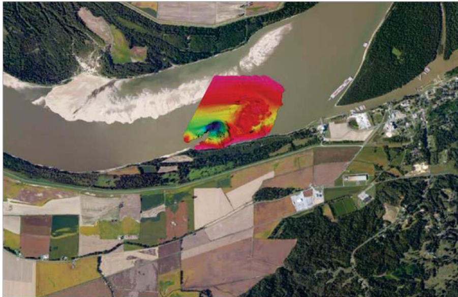
Figure 22. Scour hole (dark blue) downstream of resistant layer (higher red shades) at Hickman.
