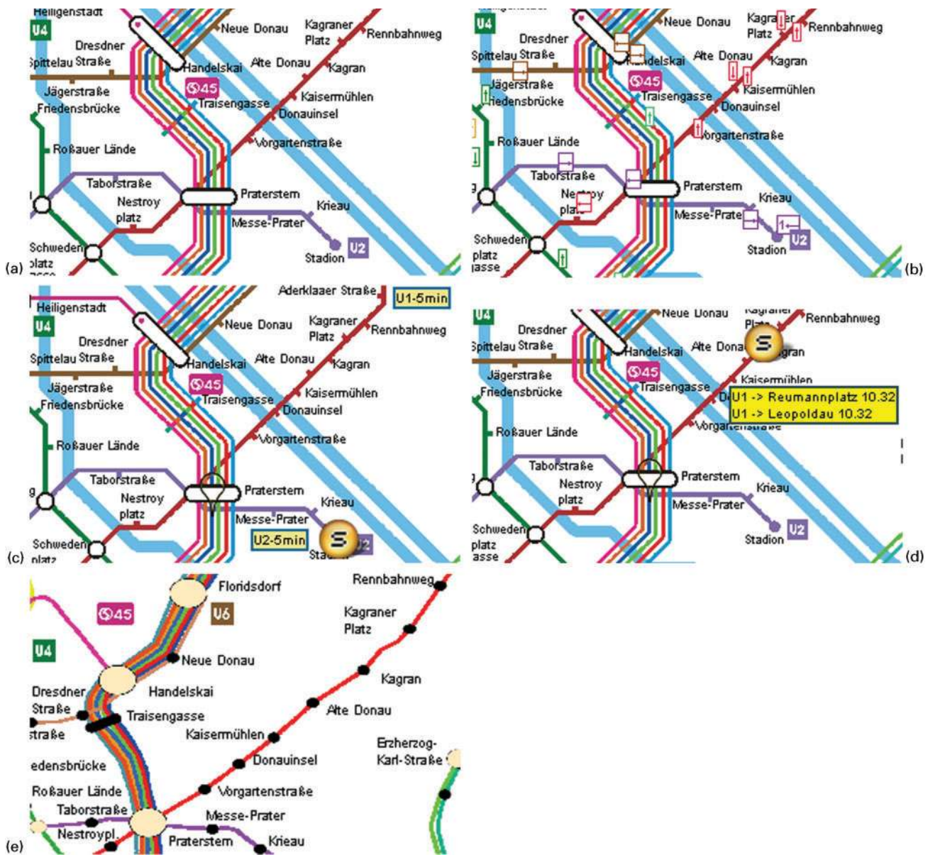
Figure 3. Five map types used in the study: (a) Schematic map; (b) Schematic map showing current vehicle positions and directions; (c) Schematic map showing headways; (d) Schematic map showing departure times; (e) Reference map
