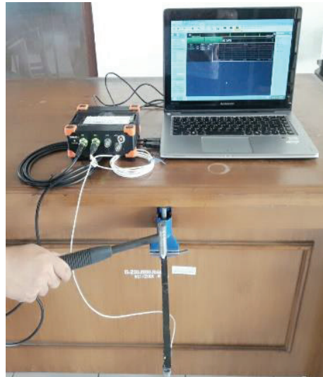
FIGURE 4. Vibration test set-up.
