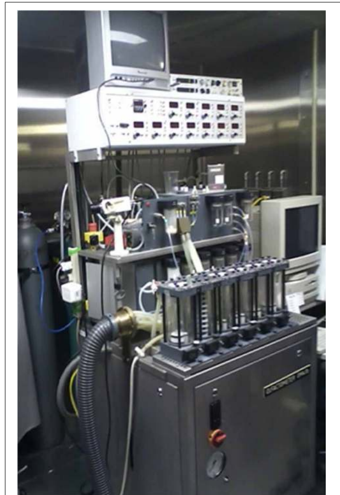
FIGURE 8 | Air-dilution olfactometer used to present pulses of odorants into a purified and humidified airstream directed through nares of a subject. This device ensures that the odor event-related potentials (OERPs) are not confounded by somatosensory artifacts due to alterations in stimulus pressure, temperature, or other factors. Photo courtesy of the University of Pennsylvania Smell and Taste Center, Philadelphia, PA.
