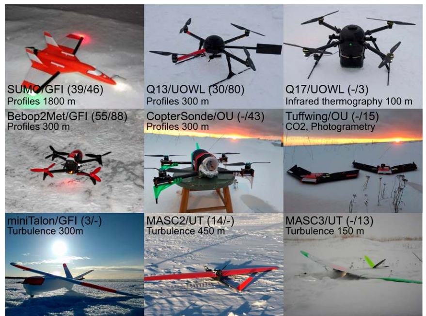
Fig. 2. The different UAS systems used during the two campaigns. The numbers of flights are indicated in parentheses for ISOBAR17 and ISOBAR18, respectively.
