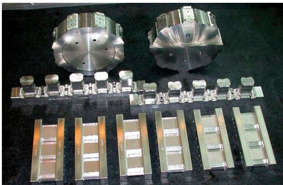
Figure 11. Tools and jigs for bracket production: the six molds, each allowing the lamination of three shells, and the contouring and finishing jigs to support the bracket during machining.
