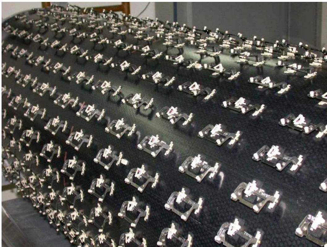
Figure 13. Barrel support cylinder complete with module support brackets.
