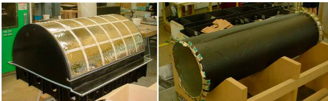
Figure 23. OTE half-shell with Pyrogel insulation and Airex stiffeners during manufacture (left) and ITE cylinder (right).
