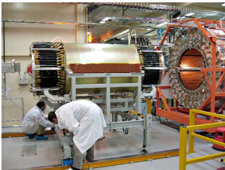
Figure 29. The SCT barrel and support cradle being set up for its transfer on the cantilever tool.
