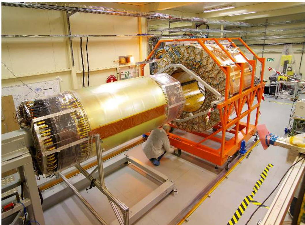
Figure 32. Translation of the TRT barrel inside the trolley over the SCT barrel.
