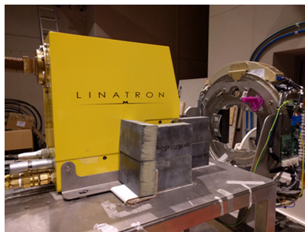
Figure 4. Fixed gantry linatron with multileaf collimators (MLCs) (white arrow) outside the magnetic resonance imaging faraday cage. The bore is positioned that the main magnetic field is aligned parallel with linatron beam.
